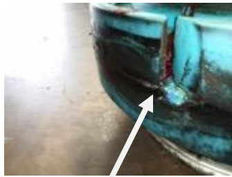
Cracks in RunFlat segment
