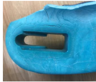
Deep cracks in RunFlat segment
