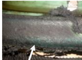
Significant wear on outside surface
