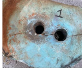
Cracks near the fixings
