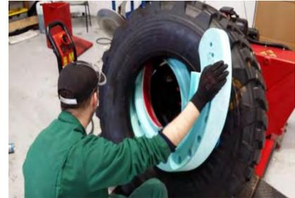
Mount tyre and Runflat system on to wheel rim and inflate the tyre, making sure the back bead is over the safety hump. (**FIG 7**).
