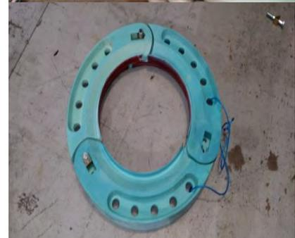
Insert RunFlat segments in to tyre, wedge slot upper most, making sure wedges sit at top of wedge bolts. (**FIG 6**).
