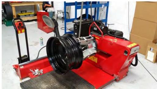
Fit metal clamp-in valve to wheel rim.
