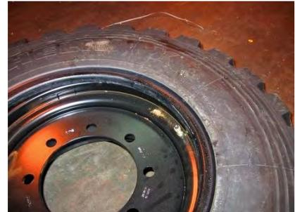
Grease undersides of RunFlat segments, making sure grease slots are completely full of grease (FIG 3).
