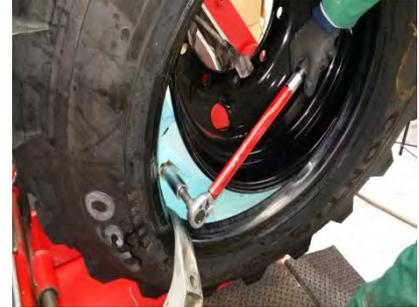
Apply Loctite to clamping plate bolts and fit clamping plate bolts at each joint position making sure double locking washers are under the head of each bolt. (**FIG 12**). Tighten down each clamping plate bolt to maximum torque with standard wrench (**FIG 13**).
