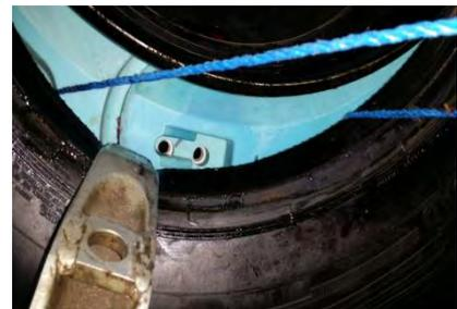
Apply Loctite thread adhesive to wedge bolt and insert into *TSI* system making sure double locking washer is under the head of the bolt (**FIG 10**). Tighten down wedge bolt so that the wedge top is level with the top of the *TSI* system (**FIG 11**). Remove the assembly cord after the final wedge bolt has been fitted.
