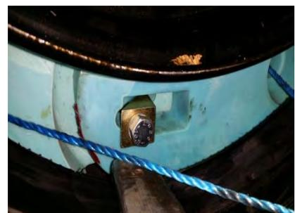
Tighten down the wedge bolts in turn so that the top of each wedge sits just below the top of the *TSI* system. Use Torque wrench to tighten each wedge bolt to a minimum torque setting of a 25Nm -Max 30Nm (**FIG 11**).
