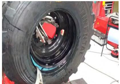
Using the tyre machines lifting arm pull top bead of the tyre to expose the open joint and using the cord, pull ends of *TSI* together (**FIG 9**).
