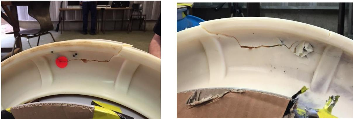
RunFlat International carried out similar shooting tests at -20°C, +20°C and +50°C, with the same outcome: no macro cracks at either end and an exit hole which is hardly apparent as the material tends to heal following the passage of the bullet.
