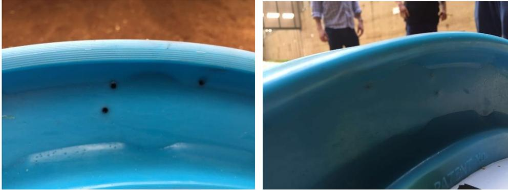
The photos above show the entry (left) and exit (right) holes of three 7.62 NATO bullets shot from 50m (as per FINABEL) within a 25cm<sup>2</sup> surface: no visible cracks at either end which would otherwise propagate rapidly in run flat mode.
